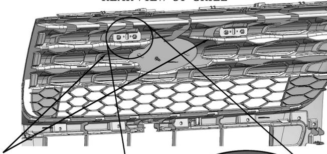
2. Remove both grill inserts by carefully pinching the two clips that secure each of them.
